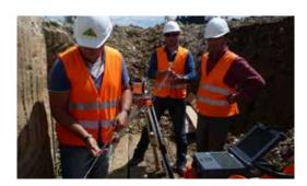
Cross hole sonic logging provides a full and thorough investigation of the quality and consistency of concrete bored piles.
